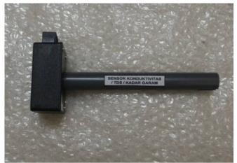
Figure 5. TDS Sensor/Conductivity
