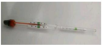
**Figure 1.** Hydrometer Salinity
