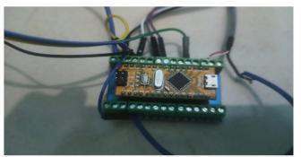
Figure 9. Arduino nano 328 system
