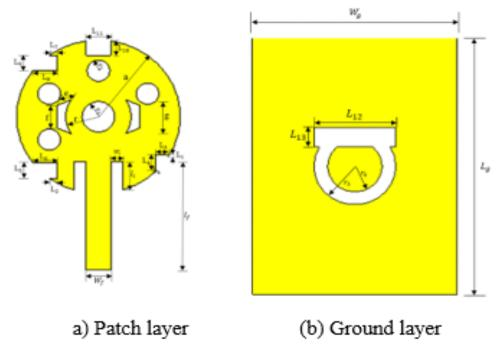
Figure 2. The Geometry of the Improved Proposed Antenna, (a) Patch Layer, (b) Ground Layer
