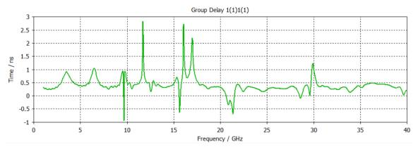
Figure 5. The group delay values versus frequency
