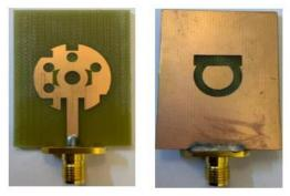
a) Patch layer (b) Ground layer Figure 6. The Geometry of the Fabricated Proposed Antenna, (a) Patch Layer (b) Ground Layer
