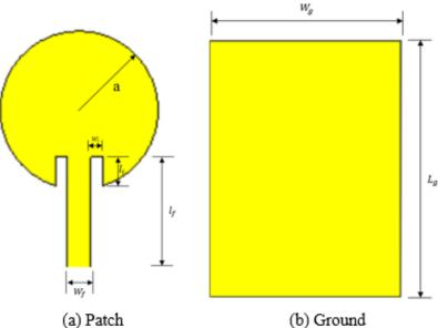
Figure 1. The Initial values of the designed patch antenna, (a) patch layer (b) ground layer
