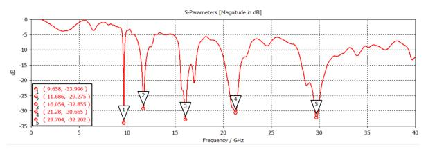
Figure 3. The reflection coefficient ( $S_{11}$ ) versus frequency
