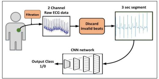
Figure 1. Workflow architecture of proposed method
