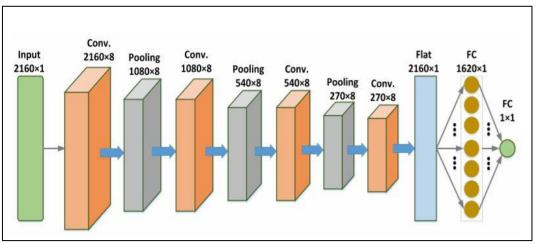
Figure 2. Proposed CNN architecture
