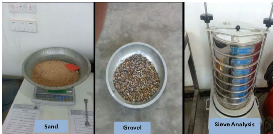
(a) Sieve Analysis &amp; Mixing
