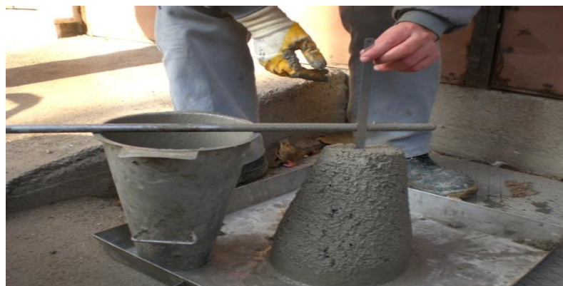
(b) Workability Test
