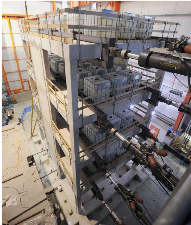
Figure 4. Barrels of water used within the structure
