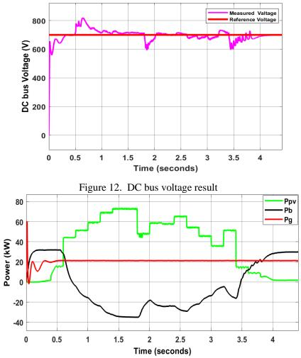
Figure 13. Power curves of the battery, PV and grid at varied solar irradiation case
