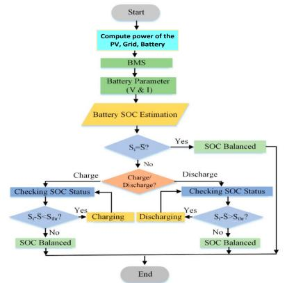
Figure 7. It proposed PMS algorithm of the hybrid PV-battery inverter
