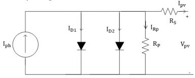
Figure 3. Two-diode PV cell model
