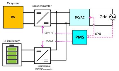
Figure 3. Proposed PV-battery grid connected inverter
