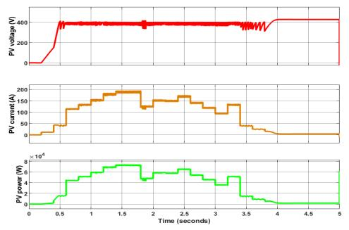
Figure 11. Results of the PV system from top to bottom: voltage, current and power
