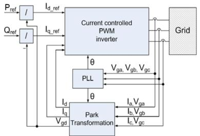
Figure 8. PQ control method for VSC inverter
