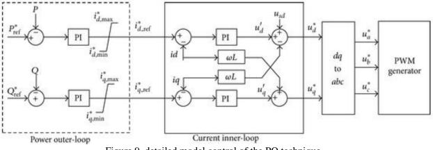
Figure 9. detailed model control of the PQ technique
