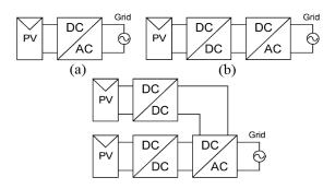
Figure 1. PV inverter architectures-based power stage unit (a) single stage inverter (b) two stage inverter (c) Multi stage inverter
