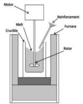
Figure 2. Stir casting principle
