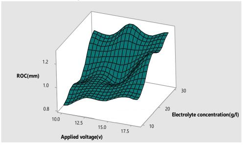
Figure 6. Relationship among radial over cut, electrolyte concentration, and voltage
