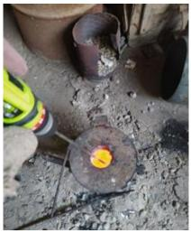
Figure 3. Stir casting process
