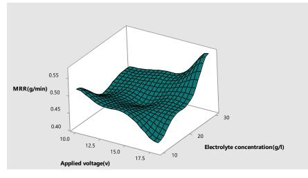
Figure 10. Relationship among material removal rate, Voltage and EC
