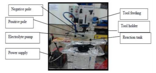
Figure 4. Electrochemical machining
