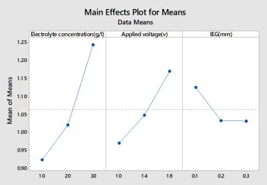
Figure 5. Influence of electrolyte concentration, voltage, and IEG on the ROC
