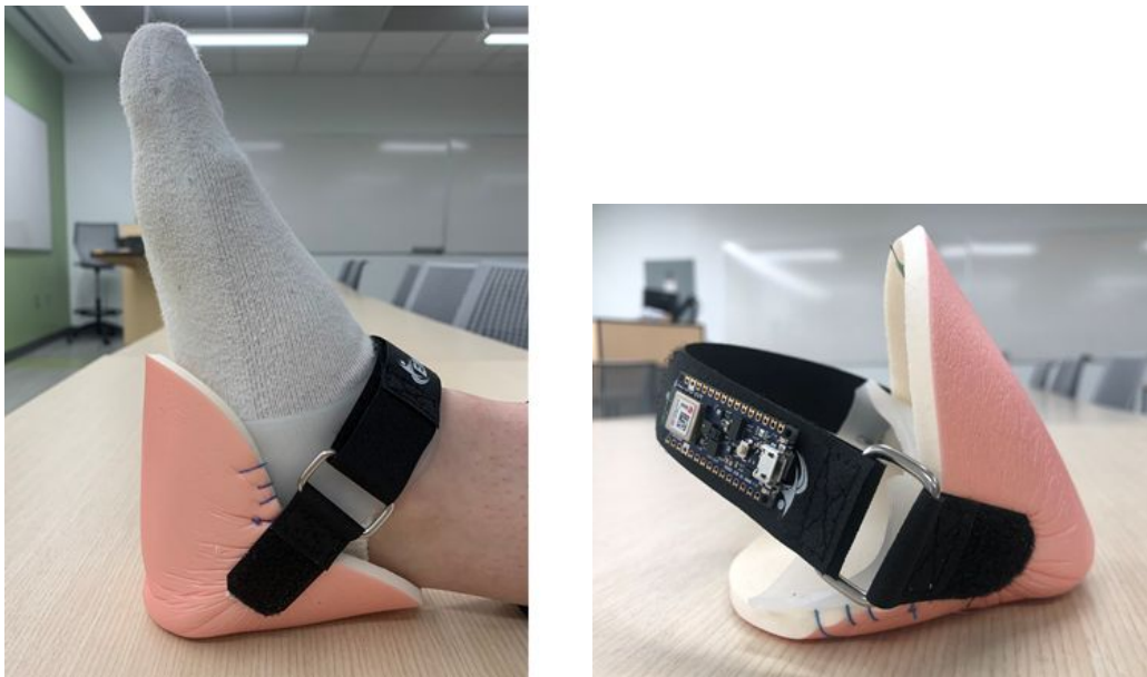
Figure 8. Form factor prototype using silicone foam dressing designed for the heel.
