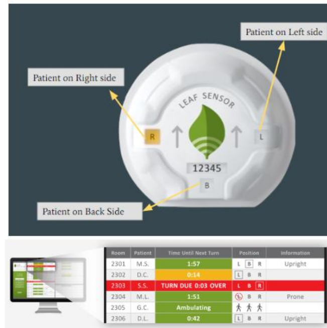
Figure 1. The Leaf sensor is a disposable, wireless stick on sensor that provides information about the patient's mobility to a computer interface [19].
