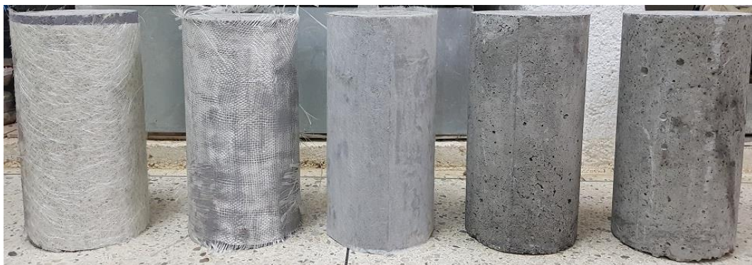
Fig. 8 – Reinforced and unreinforced Concrete columns
