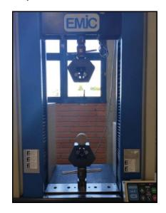
Figure 4. Diametrical compressive strength test equipment.
