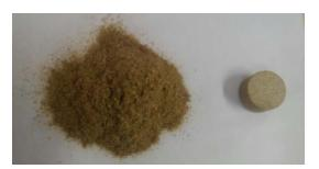
Figure 1. Same weight of biomass in bulk and compacted format, respectively.
