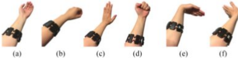
Figure 1. Human hand-over intentions for human-robot collaboration by [25]: (a) to need; (b) to give; (c) to stop; (d) to continue; (e) speed up; (f) slow down
