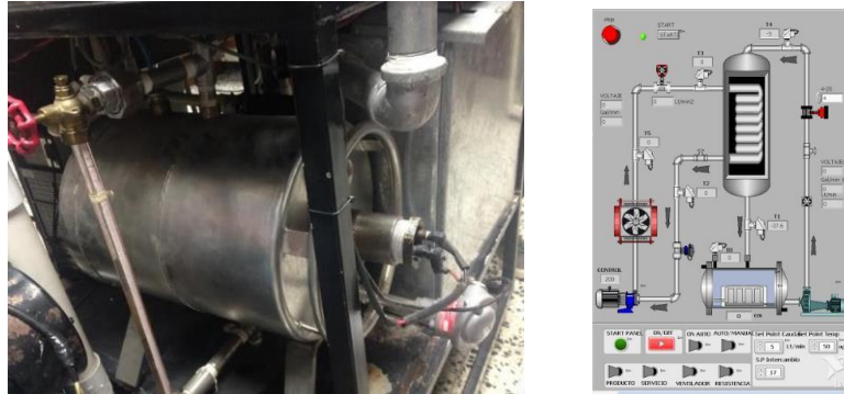
Figure 20. Graphical interface for thermal plant control.
