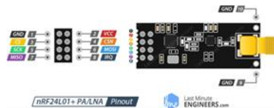
Figure 10. The pin diagram of the NRF24L01 Antenna is shown. [18]
