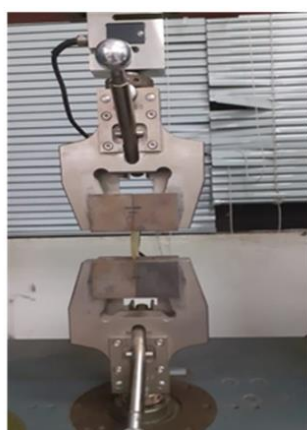
a. UTM (Universal Tensile Machine) “Zwick Roel”
