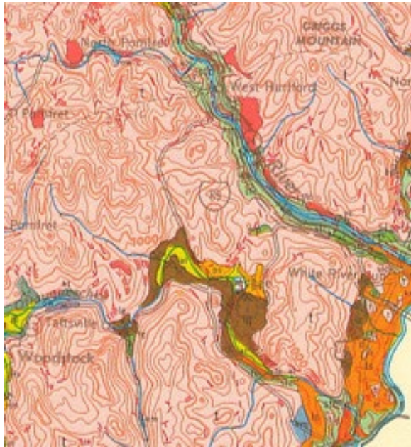
Figure 2. Surficial geologic map showing sediments in lower White River watershed (middle to upper right) near the confluence with the Connecticut River. Green unit labeled STC is adjacent to Route 14 where samples were collected for analysis. Adapted from Doll, 1970.
