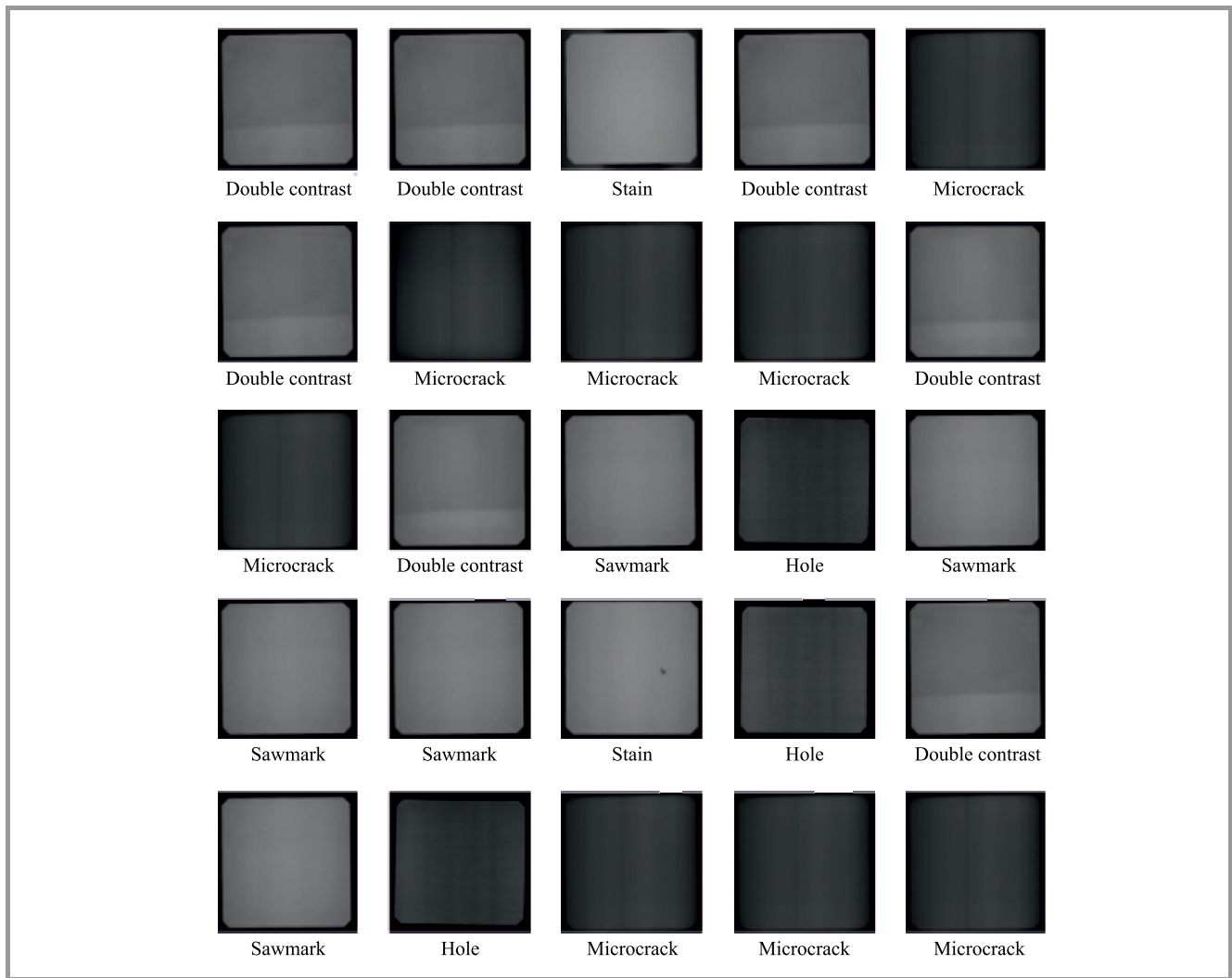
Fig. 5. Sample of defect classification prediction results of 25 images from the testing set.
