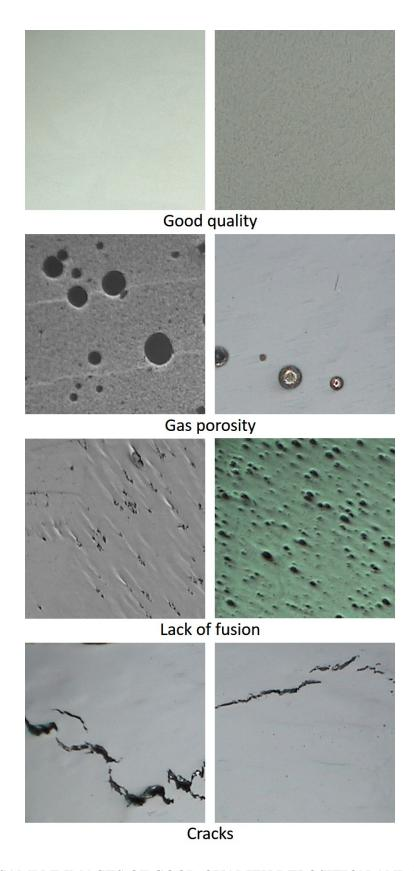
Figure 1. SAMPLE IMAGES OF GOOD QUALITY DEPOSITION AND DEFECTS.
