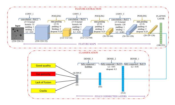
Figure 3. FINAL CNN ARCHITECTURAL SETTING AND PARAMETERS FOR THE DEFECT DETECTION OF AM PARTS.
