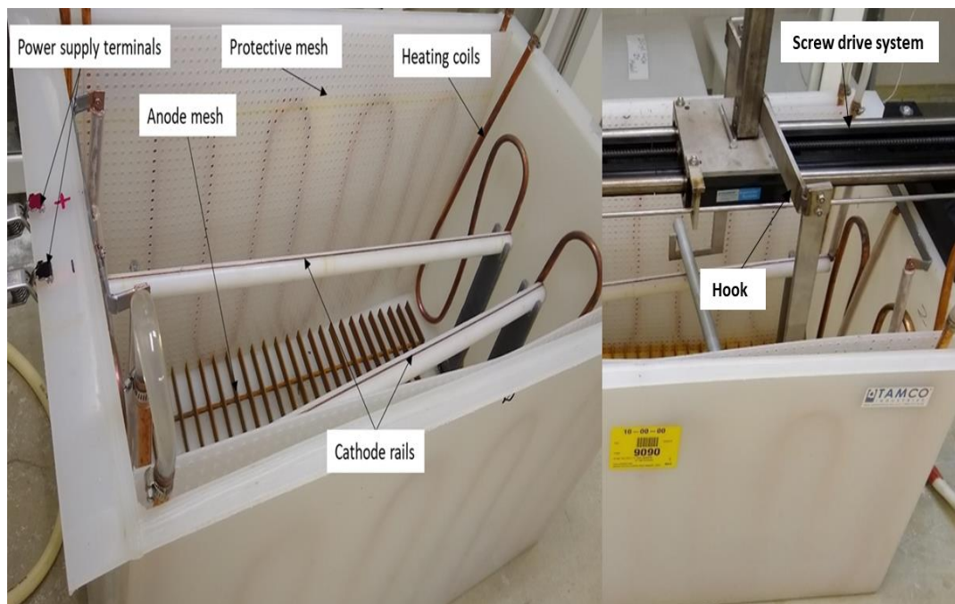
Figure 3. Laboratory tube plating cell.
