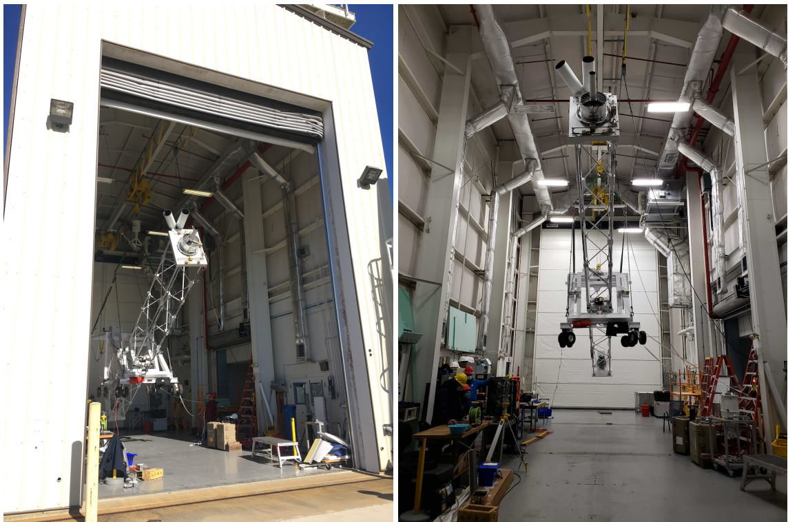
Figure 2.1. The WASP platform with the XL-Calibur mission science hardware mounted as the centerbody is shown in suspended system flight functional configuration at NASA WFF.
