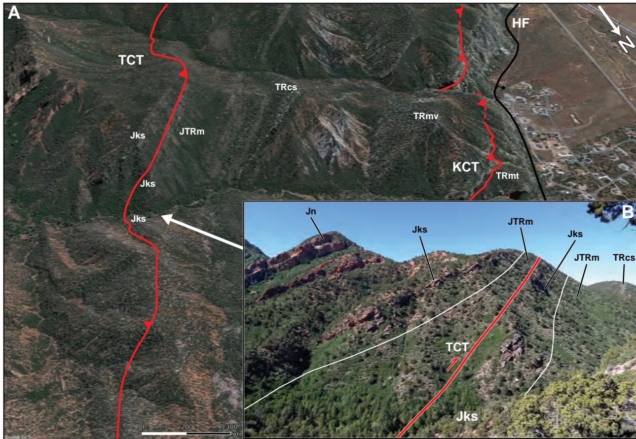
Figure 17. The Taylor Creek thrust at Camp Creek. A) Google Earth 3D terrain view south into Camp Creek showing the Taylor Creek thrust duplicating the Springdale Sandstone Member of the Kayenta Formation and the Dinosaur Canyon Member of the Moenave Formation. B) Edge-on field photo of the Taylor Creek thrust duplication.
