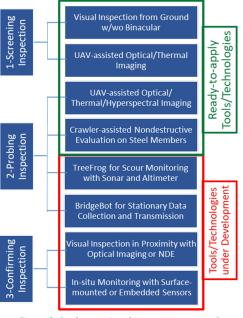
Figure 3: A robot-assisted inspection protocol.
