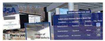
Figure 4: Hand-free bridge inspection enabled by AR.
