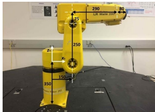
Figure 7. Photograph of FANUC LR Mate 200 i robot side view with links lengths (mm).
