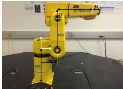
Figure 8. Photograph of FANUC LR Mate 200i robot side view with links lengths.
