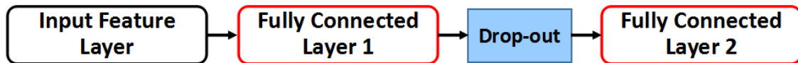
Figure A3.6. The architecture shared by CNN_2^6 in the second layer and CNN_3^7 in the third layer. In CNN_2^6 , the input feature layer contains the high-level appearance feature, which is extracted from the 4 key moments. In CNN_3^7 , the input feature layer consists of visual and temporal information.
