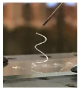
Figure 4.18. Free-Standing Spiral Deposited with Fiber-Fed Process
