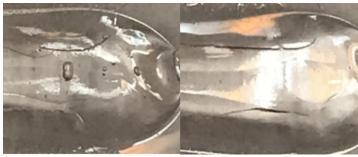
Figure 3.16. Borosilicate Track Scanned with Gaussian Beam (left), Quasi-Uniform Intensity Beam (right)
