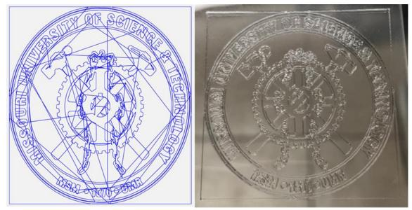
Figure 4.14. Path Generated to Deposit S&T Cog (left) Deposited Soda-Lime S&T Cog Pattern (right)
