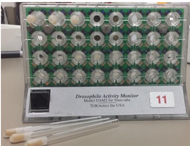
Figure 2.2. Drosophila Activity Monitor used to record activity in individual flies for every minute.
