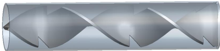
Figure 2.11. Diagram of full length twisted tape with oblique teeth
