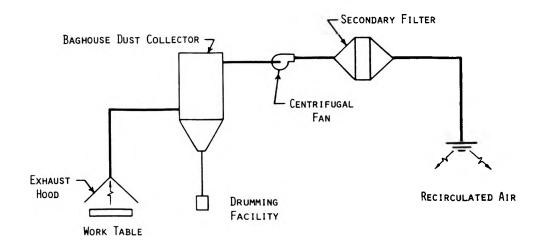
FIGURE 1. RECIRCULATION SYSTEM SCHEMATIC
