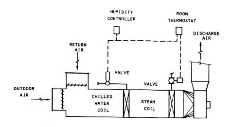
FIGURE 4. WORKSPACE AIR HANDLING SYSTEM
