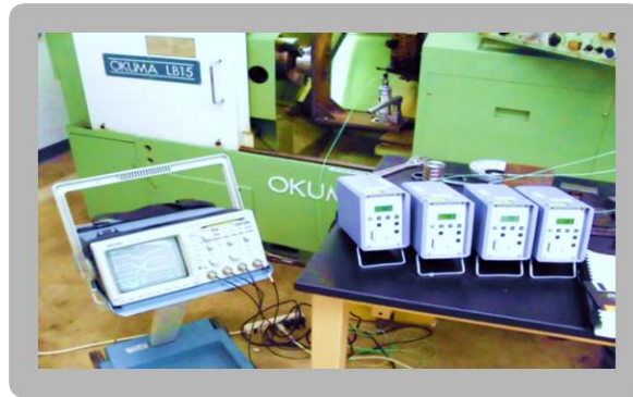
Figure 5. Set-up for the Calibration of the Load Cell
