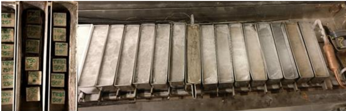
Figure 6. Test specimens in a freeze-thaw durability chamber.
