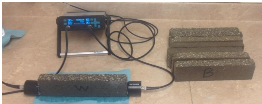
Figure 9. Ultrasonic pulse velocity test.
