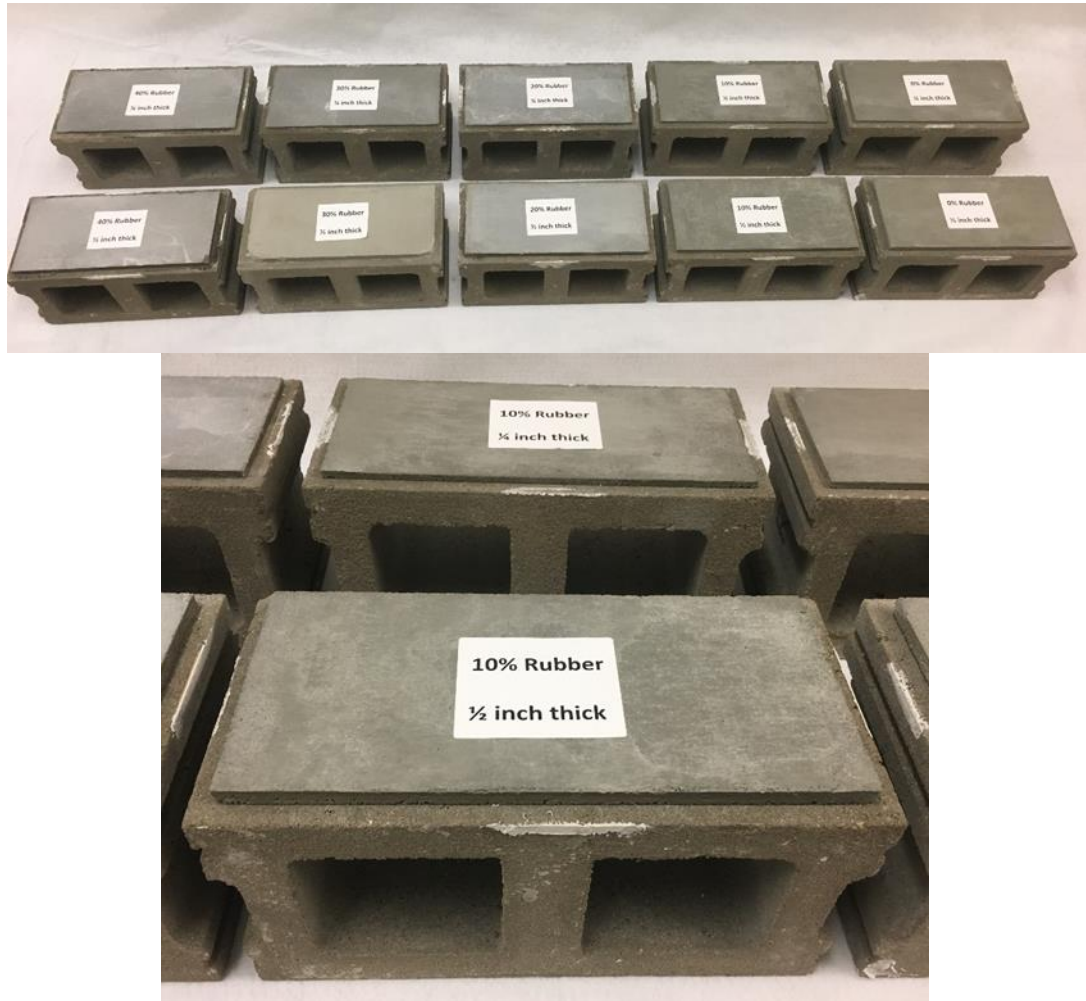
Figure 5. Different thicknesses of rubberized mortar plaster with five different ratios of RFP.
