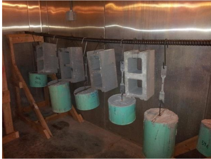
Figure 6. RCMUs in the environmental chamber.
