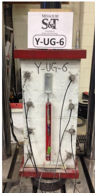
Figure11. Measuring strain of four blocks height masonry prism.
