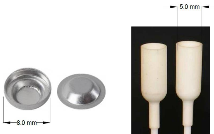
Figure 5. Standard molds for samples to test the thermal characterization of rubberized paste.
