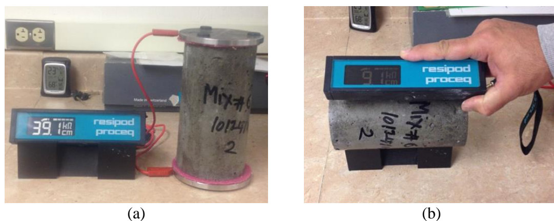
Figure 4. Electrical resistivity: (a) Bulk, and (b) Surface.
