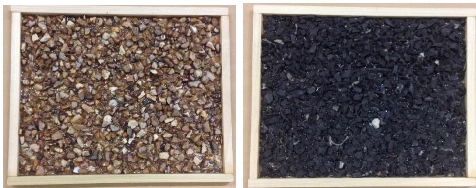
Figure 5. Chip seal specimens for image processing test.
