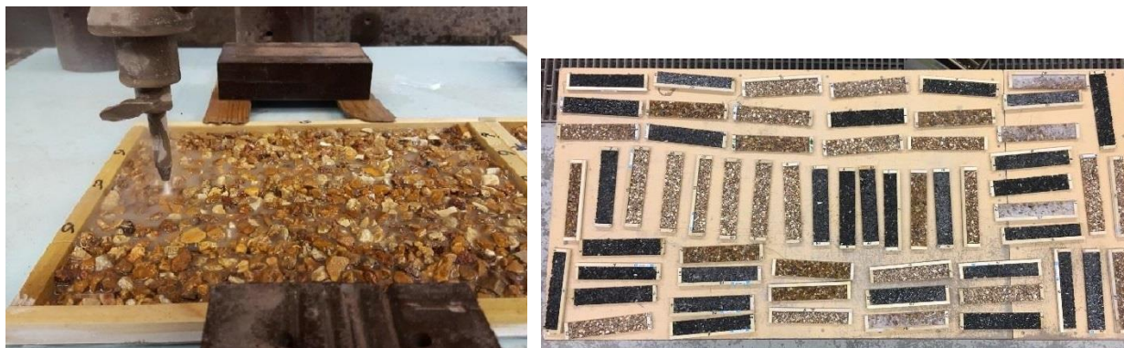
Figure 6. Sectioning the chip seal specimens using water jet cutter.
