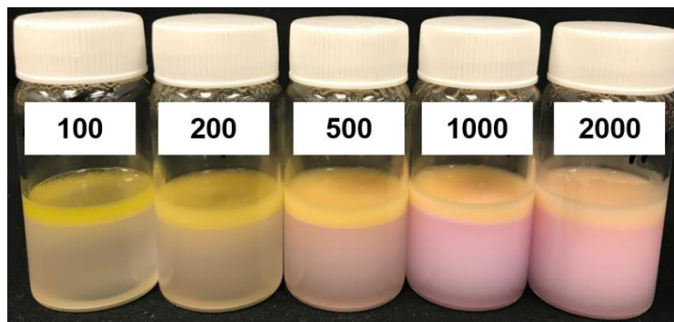
Figure 6. Decane/water emulsions stabilized by the PAM 100 MBAA 0.1 nanogels at nanogel concentrations from 100 to 2000 mg/L.
