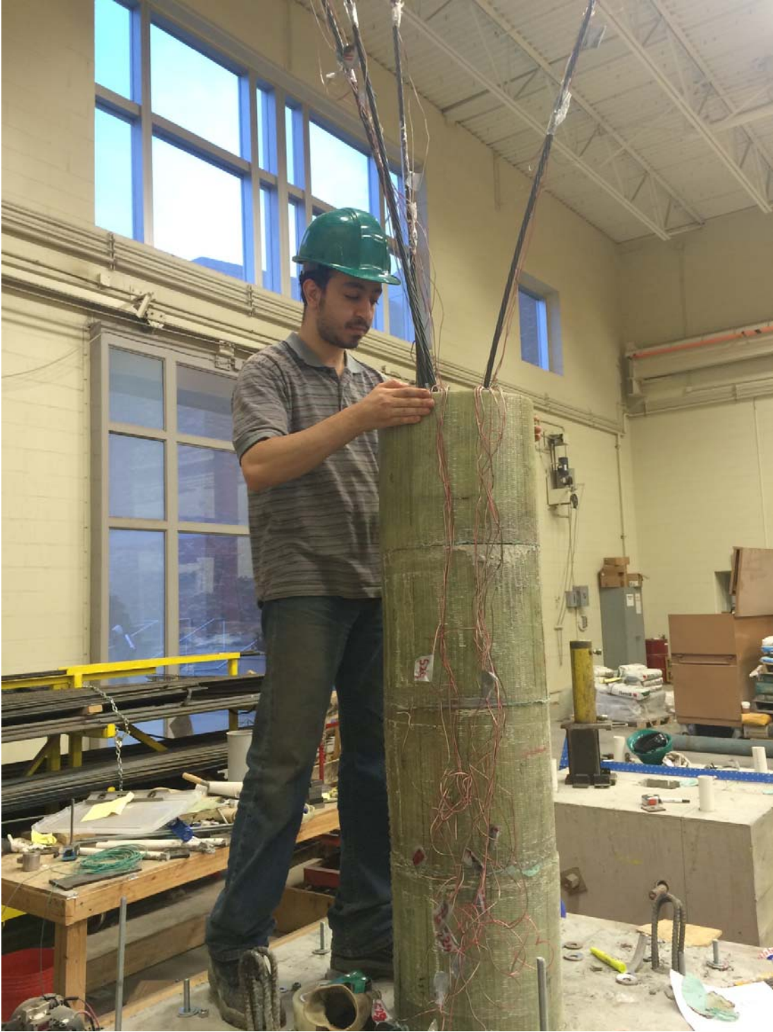
Figure B.6. Construction of the segmental column
