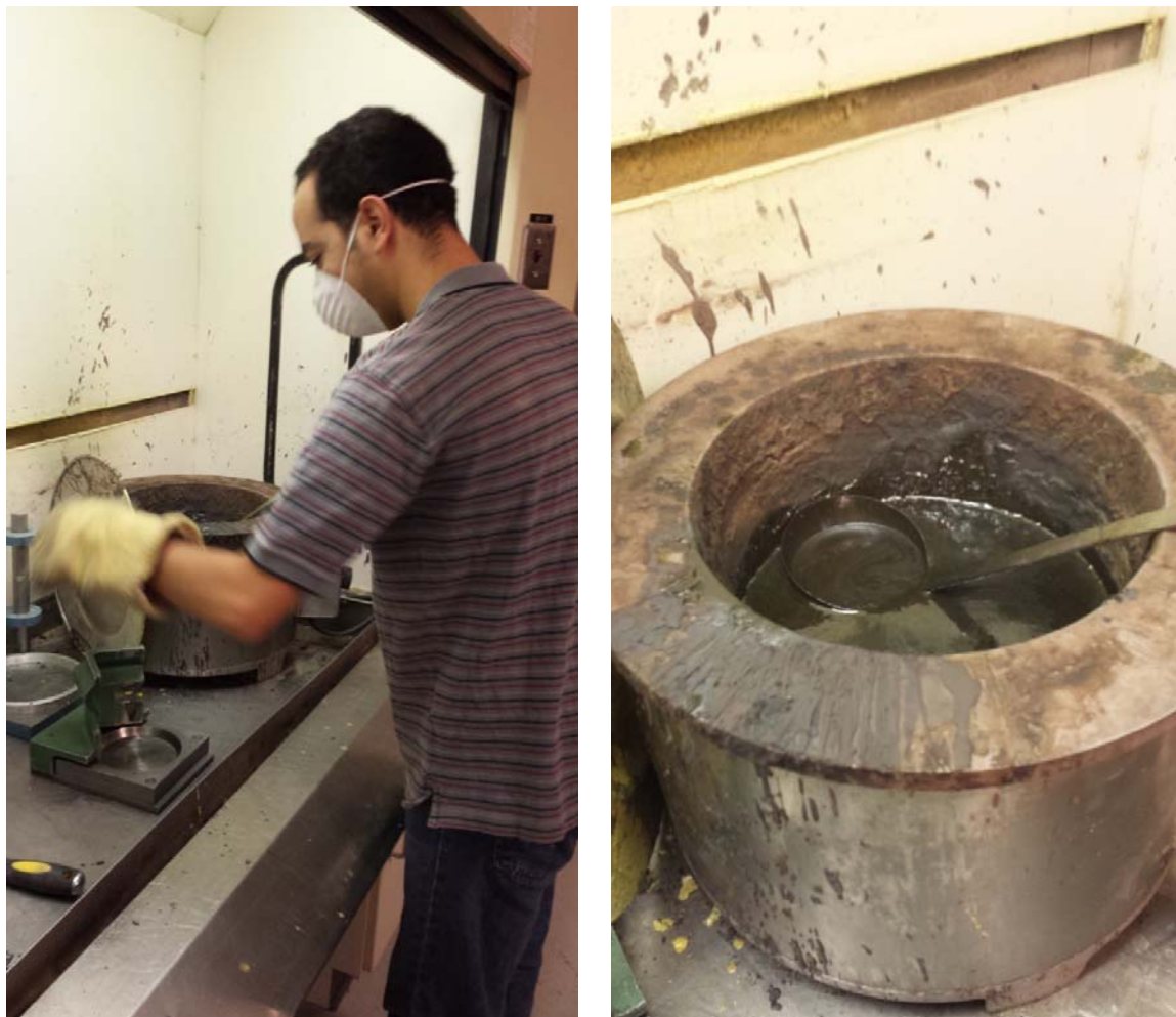
Figure A.1. Sulfur capping preparation for the cylinders
