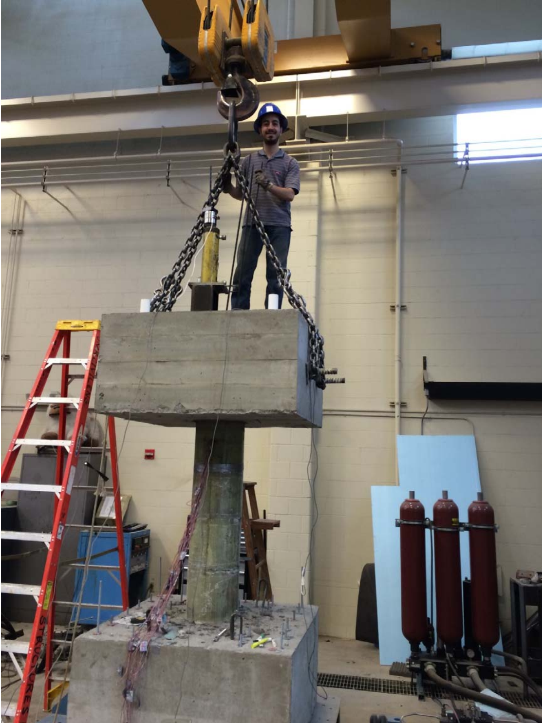
Figure B.7. Post-tensioning of the segmental column
