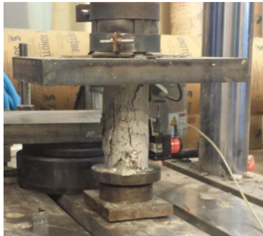
Figure 3. Compression test setup.
