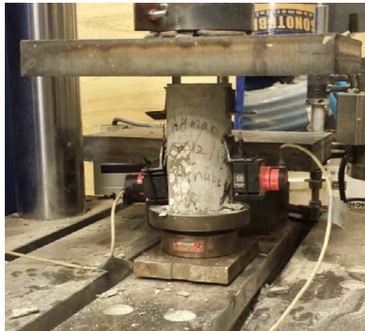
Figure 2 -- Compression test setup
