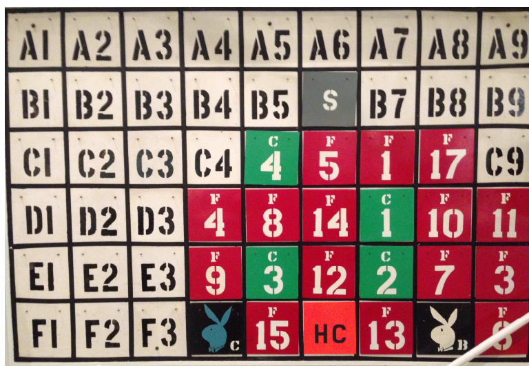
Figure 3. Picture of the MST reactor core grid plate. Rabbits represent experimental facilities (Cadmium and Bare), an “F” above the number represents a fuel assembly, a “C” above the number represents a control rod, “HC” is the hot cell and “S” represents a source for reactor start-up.
