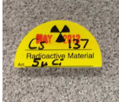
Figure 3. The ^{137}\text{Cs} source used in the deadtime – temperature and fatigue dependence measurements.
