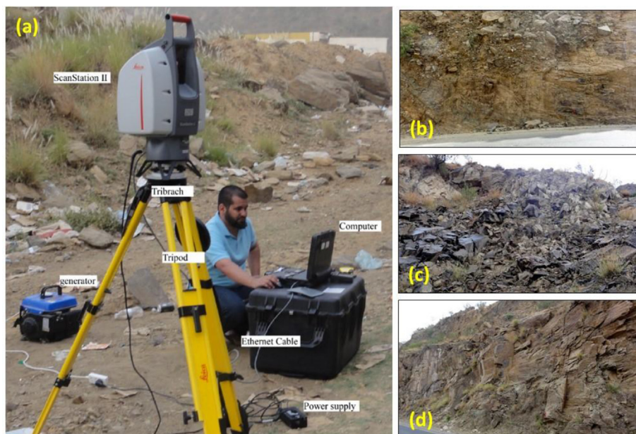
Fig. 2. (a) The equipment used for data collection, (b), (c), and (d) sites A1, A2, and A3, respectively.
