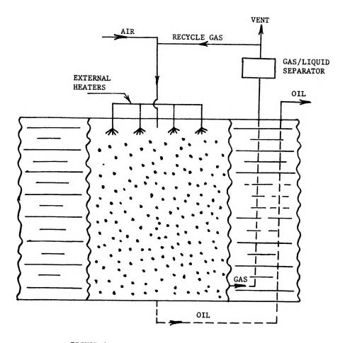
FIGURE 1. MODIFIED IN SITU OIL SHALE RETORTING
