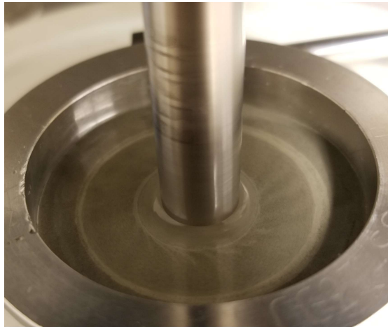
Figure 10. Bleed water at the top can be observed during test without homogenizing.
