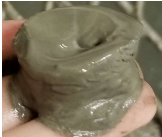
Figure 11. Plug found inside the rheometer cup after testing without homogenizing.
