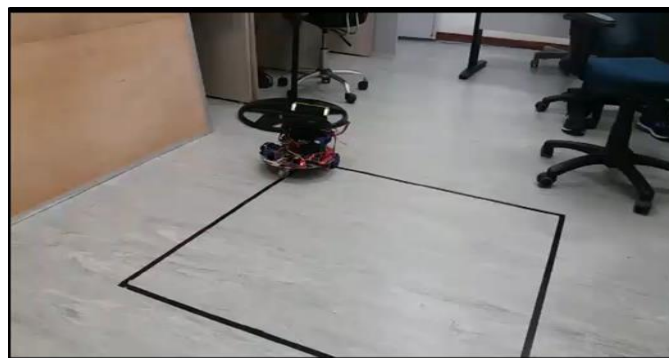
Figure 2: Path performed by the robot during the experiment. Linear and angular errors are measured at each vertex of the square
