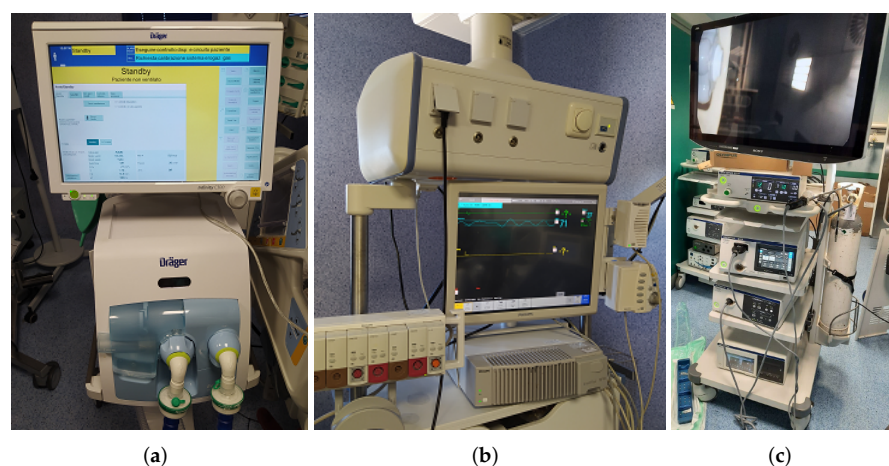
Figure 3. Electromedical devices used: (a) pulmonary ventilator; (b) patient monitor; (c) endoscope.
