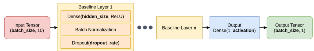
Figure 3. The Baseline architecture was used to infer the hourly sun irradiation for the 48-h forecasting. The hyperparameters tuning was set on the parameters highlighted in bold.
