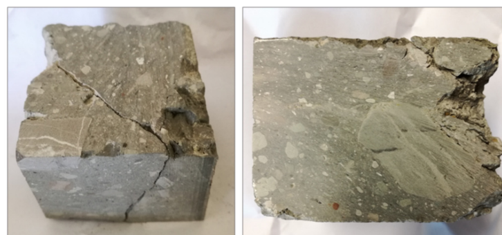
Figure 4. Mélange samples damaged during the cutting phase.
