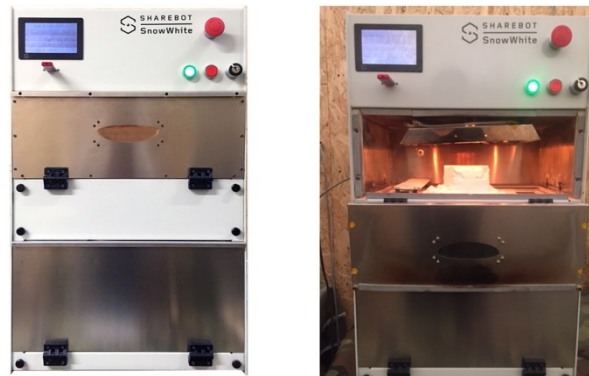
Figure 45: Sharebot SnowWhite SLS machine: external view (left image) and internal view of the build chamber (right image)
