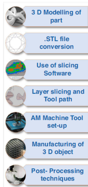
Figure 2: Flow chart illustrating all steps involved in AM file preparation and part production [12]
