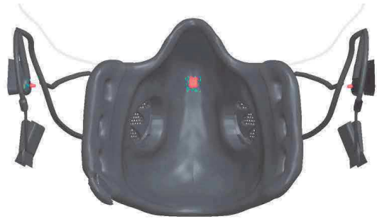
Fig. 2 Three-dimensional rendering of the AG-47 SmartMask with the positions of the main sensors highlighted in red. In the configuration shown, the mask is presented with a replication factor of 1 for the thermo-hygrobarometric (full red square) inside its facial containment cavity and with a replication factor of 2 for the intraural thermal sensors (red cones) and the pulse oximetry sensors for the ear lobe (black pliers)
