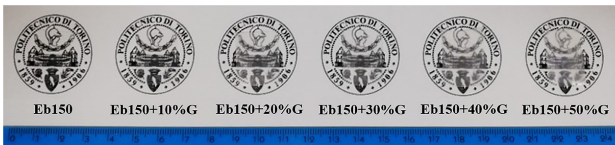
Figure 7. Pictures of UV-LED cured films prepared with different loadings of phosphate glass particles.
