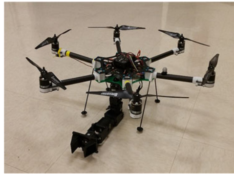
Fig. 2. Hexacopter with a three-DoF robotic arm.
