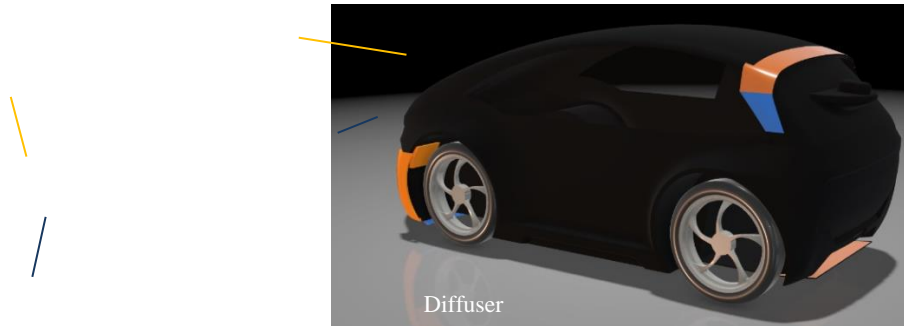
Figure 8 JUNO's aero pack in orange and blue
