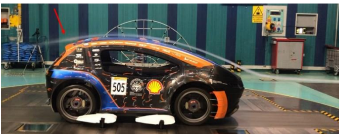
Figure 29 Complete configuration, JUNO's smoke wind tunnel test
