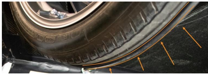
Figure 3 Rubber circumferences around JUNO's tyres
