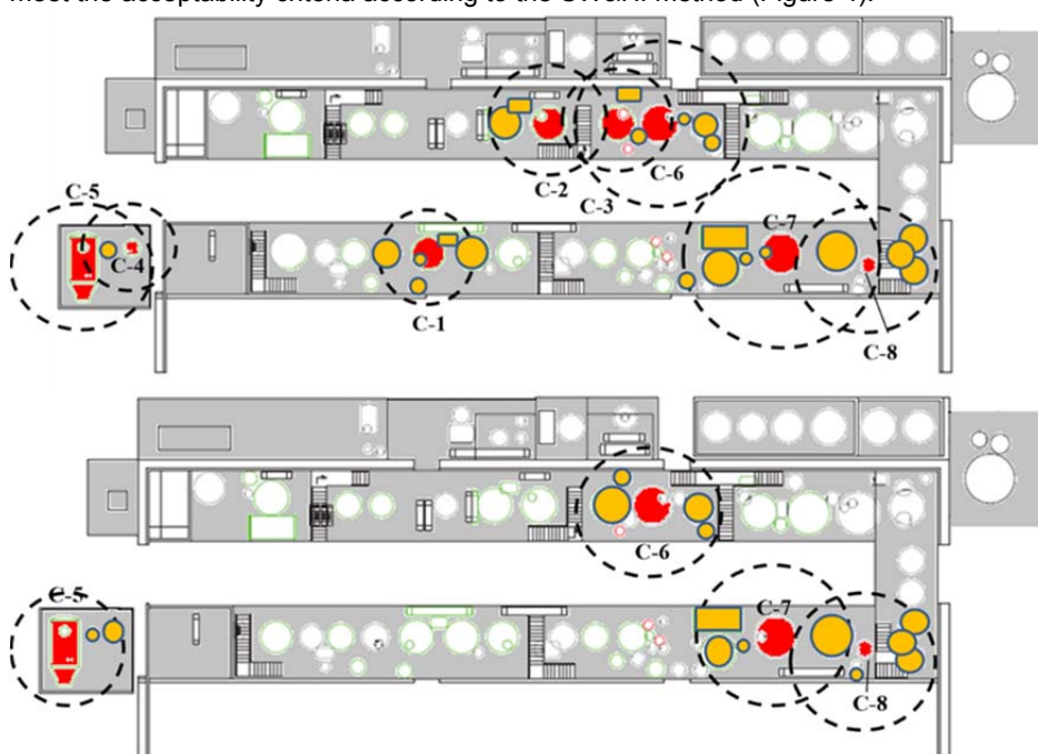
Figure 5: Graphical representation of SW&HI damage area, before (top) and after (bottom) implementation of control measures, in department C (units containing flammables with greater than 5 SW&HI are depicted in red, others in yellow)
