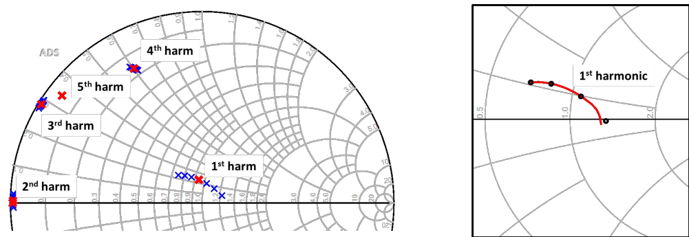
Figure 7. (Left): Spread of the S_{11} parameter with SiN thickness variations prescribed by the technology PDK. Red crosses correspond to the nominal SiN thickness of 100 nm, blue dots to \pm\sigma , \pm2\sigma , \pm3\sigma where \sigma = 2 nm [41]. (Right): Interpolated S_{11} at the fundamental frequency (red) compared to EM simulations at 4 test SiN thickness values different to the extraction ones (92 nm, 97 nm, 103 nm, and 108 nm).
