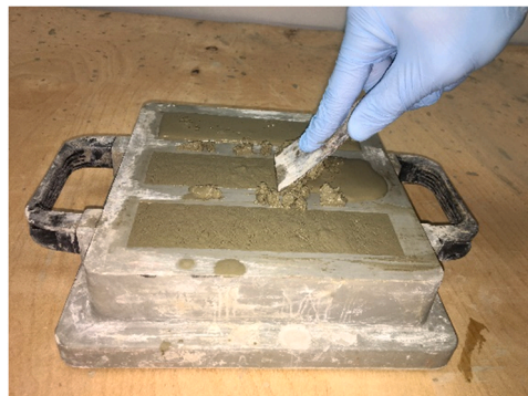
Fig. 5. Shaping phase of two-component grout samples after the casting. Mould in compliance to [31].
