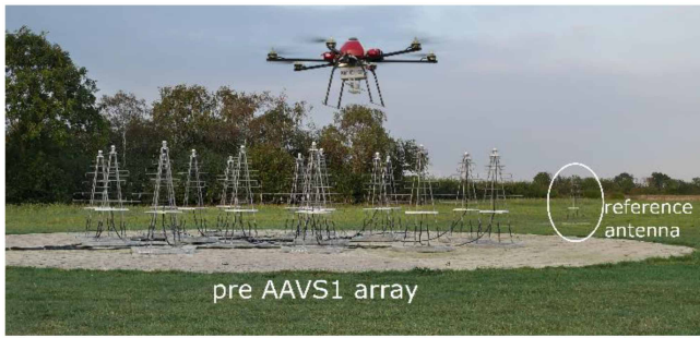
FIGURE 1. The UAV equipped with the transmitter, balun and dipole antenna flies over the array under test (pre AAVS1 array). On the right (inside the white circle): reference antenna exploited for the phase retrieval.
