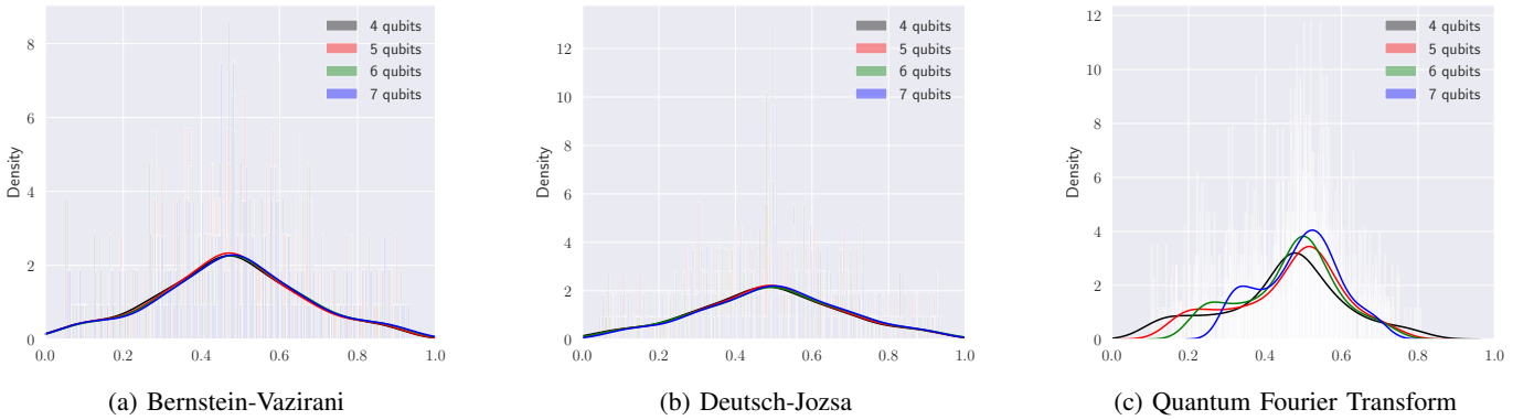
Fig. 7: Histograms of the QVF distribution of the three considered circuits increasing circuit scale. For Bernstein-Vazirani (a) and Deutsch-Jozsa (b) the number of qubits does not modify the reliability profile. For QFT (c) , the higher the number of qubits the higher the number of harmful faults.
