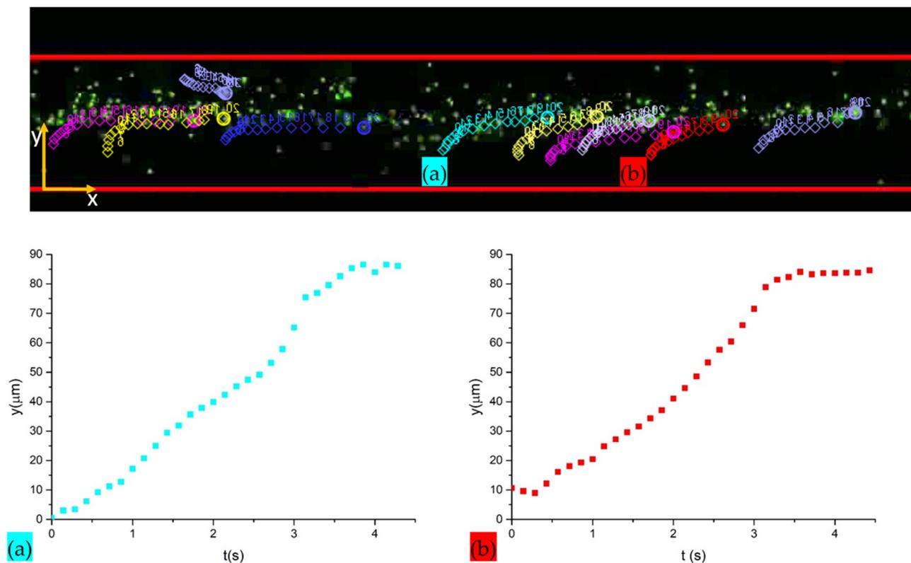
**Figure 9.** Tracking of bead paths with the Tracker 2.6 software and measurement of the transverse path  $y(t)$  from channel walls to the pressure node of two different beads (a) and (b). Measurements were performed in a specific focal plane of the  $4\times$  objective lens of the fluorescence microscope.
