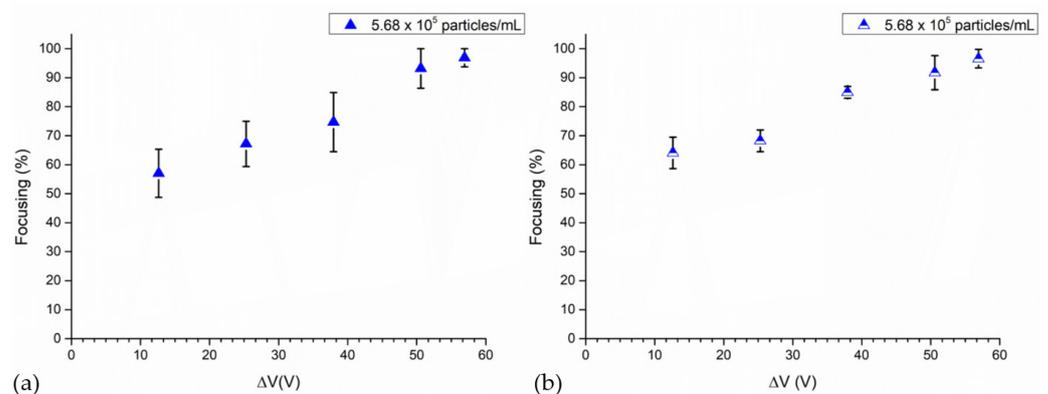
**Figure 5.** Focusing performance of the BAW device as a function of applied voltages at the transducer: (a) UV-Vis characterization and (b) image analysis. During the experiments, 4MPs concentrated at  $5.68 \times 10^5$  particles/mL were injected at 3  $\mu\text{L}/\text{min}$  into the device actuated at its resonant frequency of 4.623 MHz, while 56.92 Vpp, 50.59 Vpp, 37.95 Vpp, 25.29 Vpp and 12.65 Vpp were applied at the transducer.
