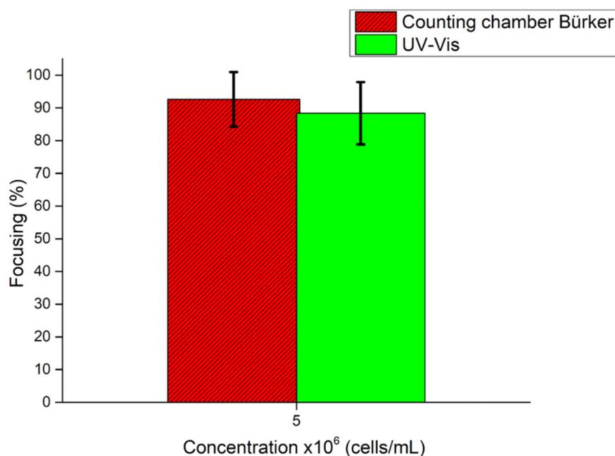
**Figure 12.** Focusing performance of the BAW device from Bürker counting chamber analysis and UV-Vis characterization. HL-60 cells concentrated at  $5 \times 10^6$  cells/mL were injected at  $3 \mu\text{L}/\text{min}$  when  $50.59 \text{ Vpp}$  was applied to the transducer, while the device was actuated at its resonance frequency of  $4.623 \text{ MHz}$ .
